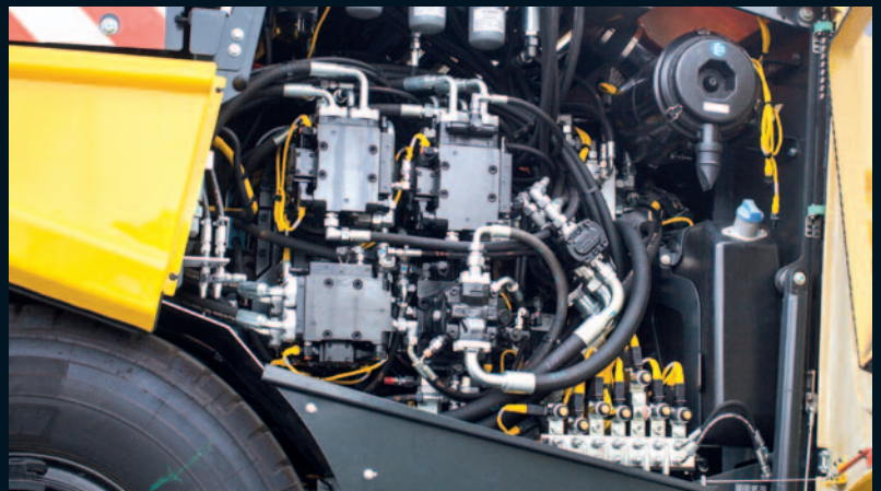
Reliable: demand-driven hydraulics deliver the exact power that is required
