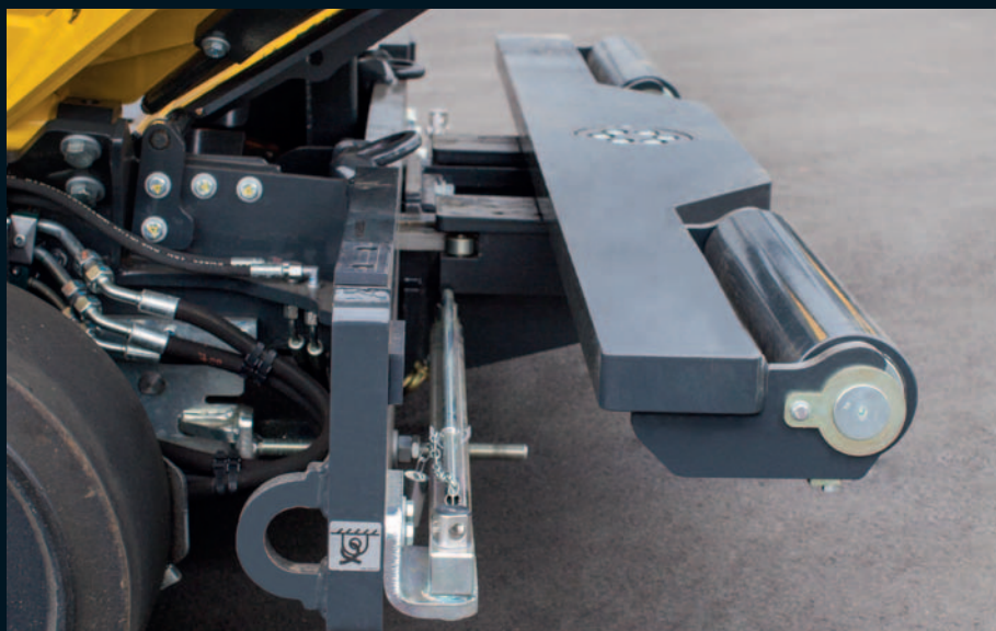
Dampened bumper rollers: hydraulically adjustable with a pendulum bearing
